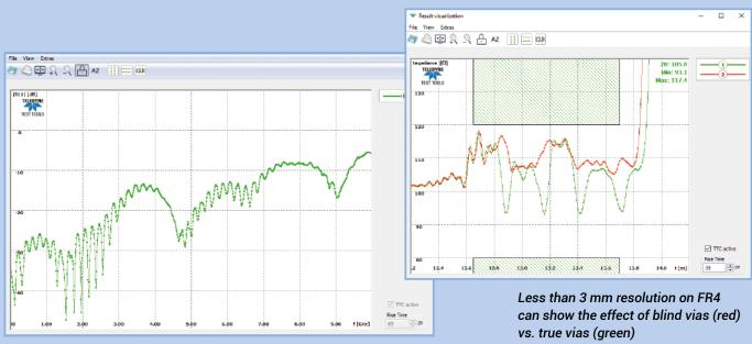
The T3SP1xD series offer S-parameter (S11) measurements up to 15 GHz
