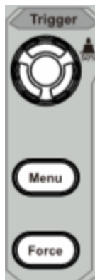
Figure 3-12 Trigger Control Zone
