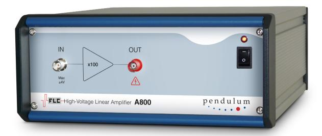
The Pendulum Instruments High Voltage Linear Amplifier A800 has a fixed amplification of 100 times and capable of bipolar high voltage output of ±400V. Any signal source with amplitude up to ±4 V can be used as an input device. The input amplitude should normally be kept within ±4 V. The A800 High Voltage Linear Amplifier is equipped with a microfuse rated at 15 mA, which will be blown if the input voltage exceeds 500% of the maximum.
