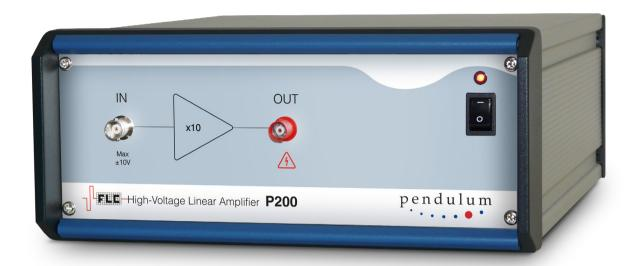
The Pendulum Instruments High Voltage High Current Linear Amplifier P200 has a fixed amplification of 10 times and capable of bipolar high voltage output of ±100V. Any signal source with amplitude up to ±10 V can be used as an input device. The input amplitude should normally be kept within ±10 V. The High Voltage High Current Linear Amplifier P200 is equipped with a microfuse rated at 15 mA, which will be blown if the input voltage exceeds 300% of the maximum.
