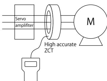
For insulation resistance measurements of industrial robots
