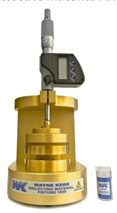
The 1020 Dielectric Material Fixture is designed to be used with the 6500B series of Precision Impedance Analyzer and 6500P series of HF LCR Meters up to a maximum frequency of 30 MHz. When used with the 6500 /K Materials Test firmware option it allows the permittivity of the Material Under Test (MUT) to be calculated automatically.
