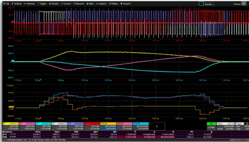
Power is measured and shown as per-cycle Waveforms for each instantaneous device switching cycle to determine operation during rotor flux changing commands.
